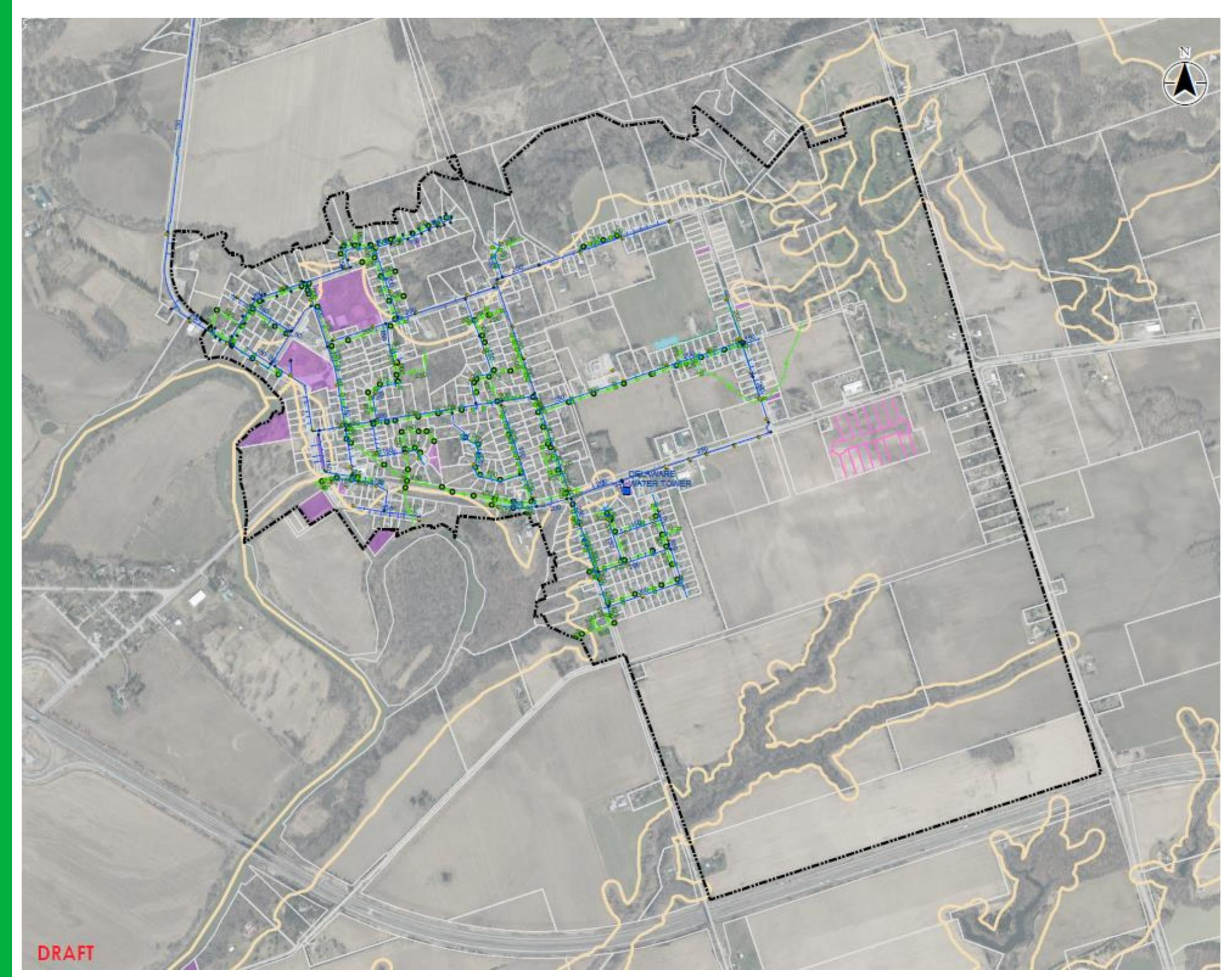
Water is provided by connection to Komoka. The community is serviced by a storage facility and a booster station.
