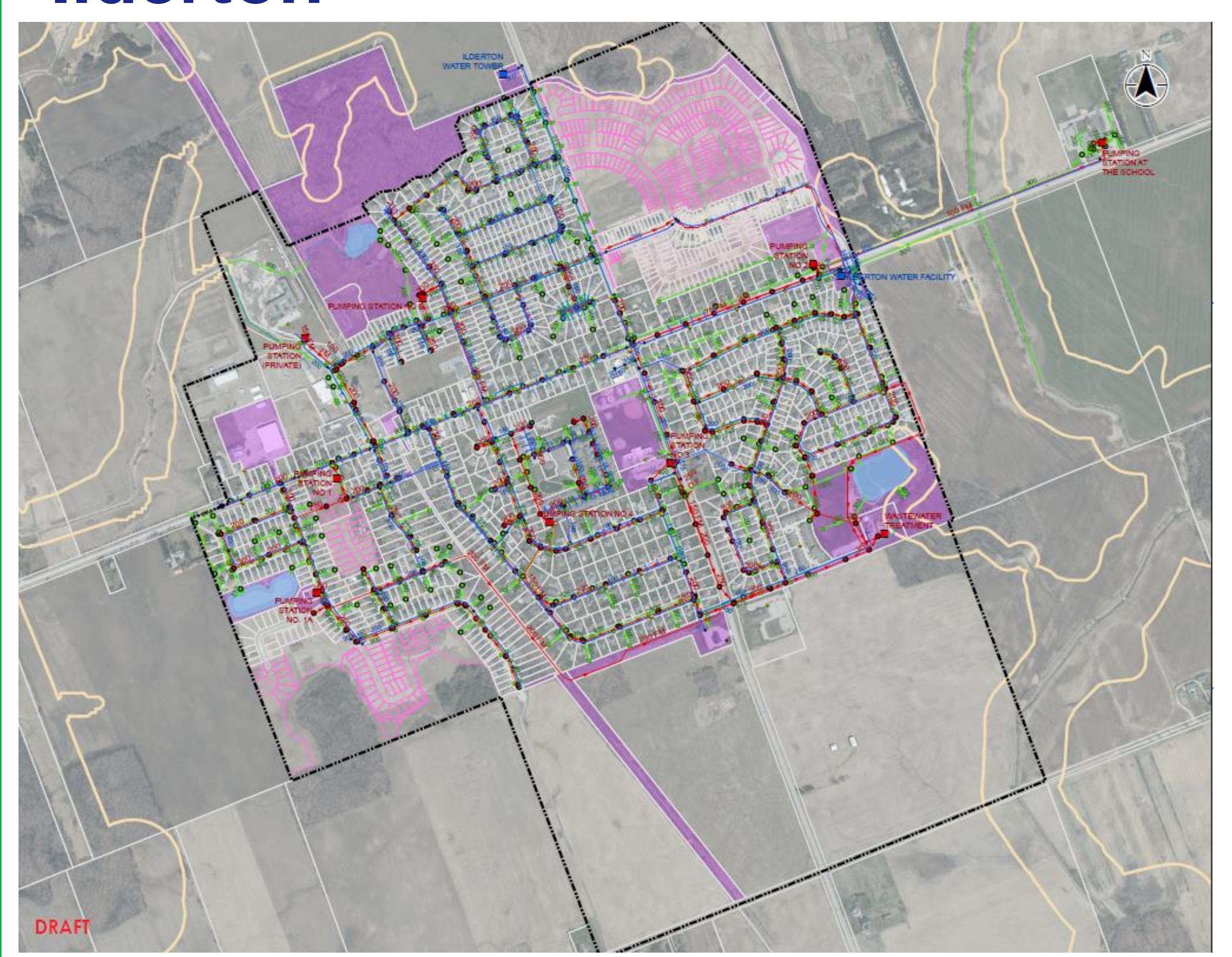
Water is provided by connection to the Lake Huron system. The community is serviced by a storage facility and a booster station.
